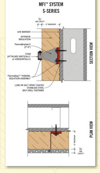
\*Lost R-Value percentage will vary based upon exact wall assembly. Values shown assume a typical 16" OC steel stud wall and 24" spacing of horizontal girts and bracket assemblies with varying thicknesses of exterior insulation.
