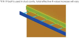
\*Base wall configuration adds R-3.3 (drywall, sheathing, air films, etc)
