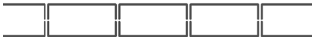
Tip-to-tip: provides cleaner, less-pronounced glass joints; for use with 41 mm flange profiles only
